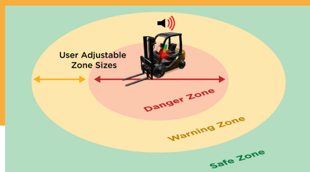
Customizable Detection Zones: user adjustable ranges for Warning and Danger Zones
