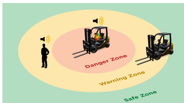
Forklift and pedestrian devices: high-level audible and/or visual alerts for direct collisions
